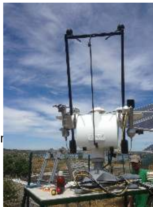
IRGASON, integrated eddy covariance system to access fluxes of momentum, energy, vapour and CO 2
