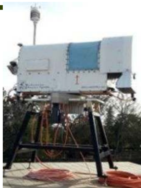
Temperature and humidity profiler
