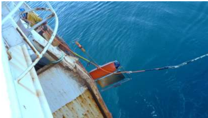
Figure 25 - Deploy of a floating port buoy with AIS antenna at top.
