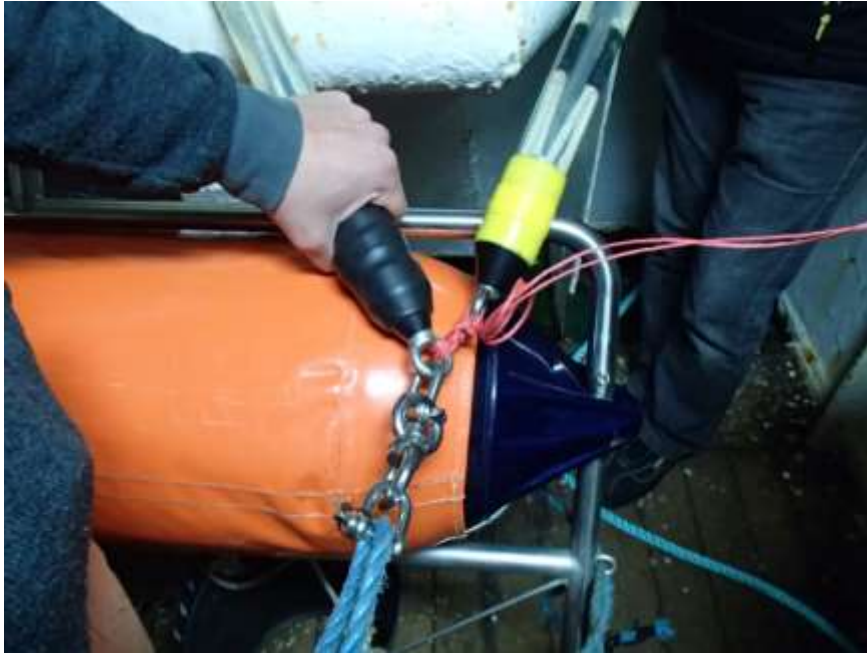
Figure 24 - The weak link joining the 2 streamers.
