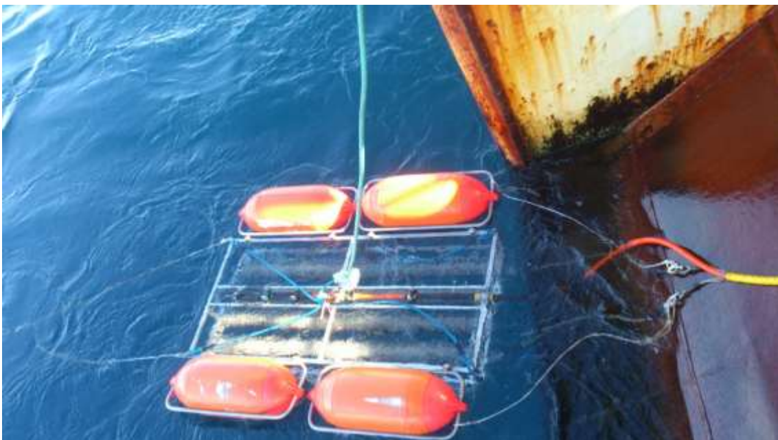
Figure 18 - GEO-SPARKER 800 seismic source.
