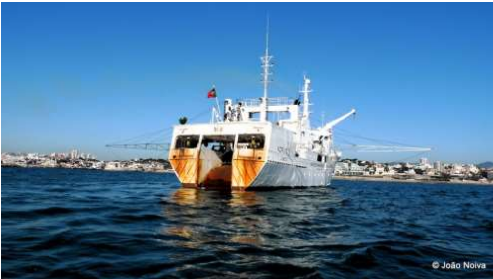
Ship Noruega, from the Instituto Português do Mar e da Atmosfera, offshore Cascais, with the two 12m outriggers mounted to tow the seismic equipment.
