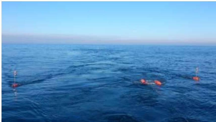
Figure 23 - The 3D towed setup. In the foreground we can see the two streamers towing buoys, which are also used to control the geometry opening. In background we can see the tail buoy where the two streamers are connected. At middle is placed the sparker source.
